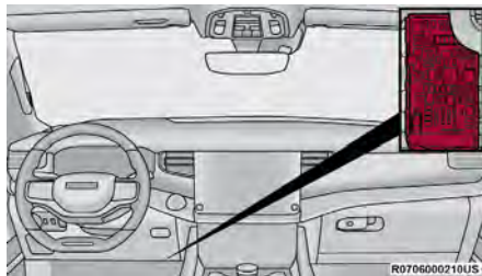
Interior Power Distribution Center Location
