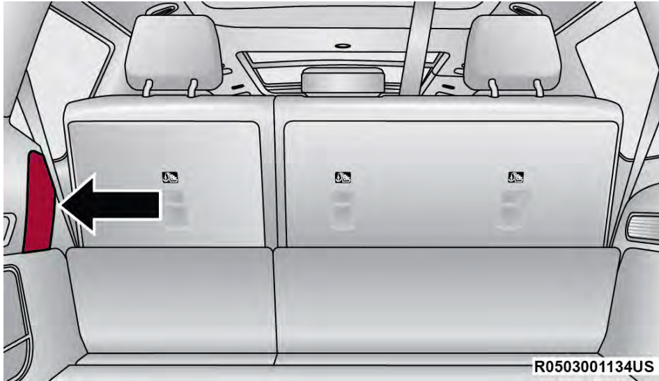
Rear Power Distribution Center Location
